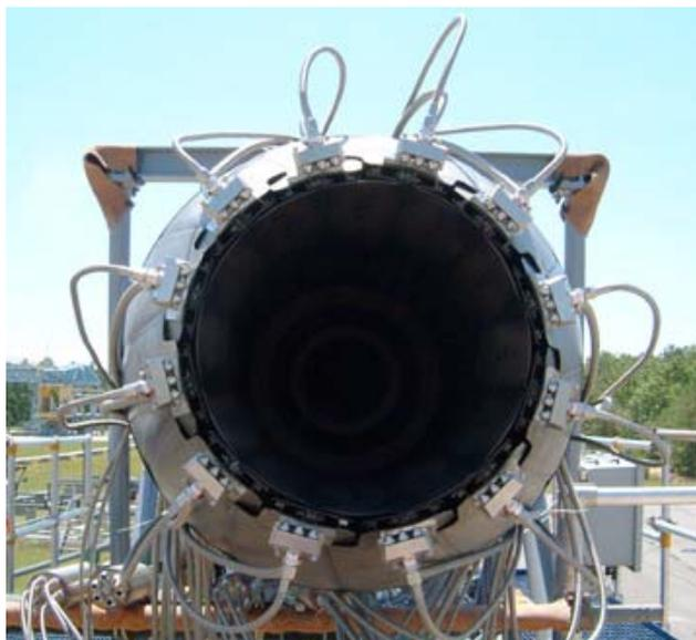
**Figure 6. F404 jet engine with the micro-nozzles installed.**
